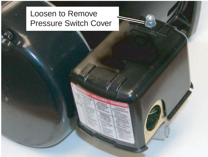
Figure 1: Pressure Switch Location
